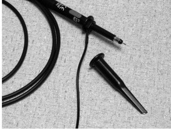
**Figure 1-4 Probe tip with grabber removed**
