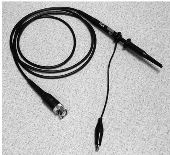
Figure 1-3 Oscilloscope probe
